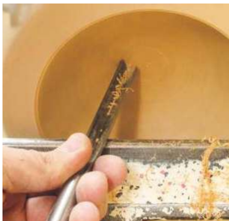
▲ Pic.31 The area of the bowl right in the middle can cause a problem as sometimes you are unable to get your normal bowl gouge in a suitable cutting position. The 60° bevel used here allows me to make small effective cuts
